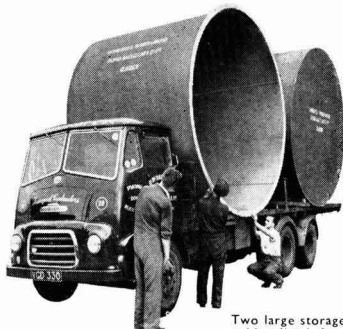
Two large storage tanks, fabricated and rubber-lined for acid manufacture by the MacLellan Chemical Plant Division.
