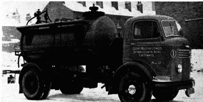
In this rubber-lined road tanker used by Godfrey Woodhead and Son for acid transport, the lining has been carried down the outside to catch any drips that may fall from the hose connection
