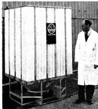
This intermediate bulk container, with capacity of 80 cu. ft. was moulded by the Engel process by Rosedale Associated Manufacturers Ltd. from I.C.I. Alkathene
