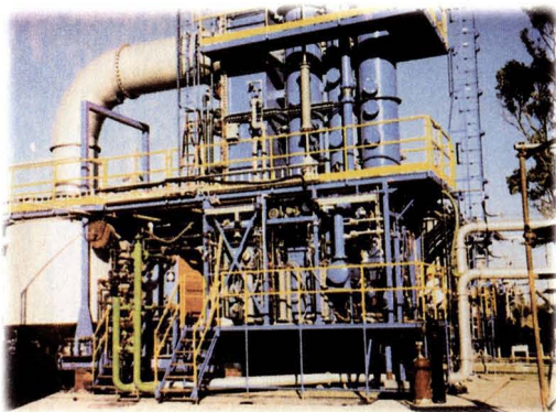
The "Destructor." Organic compounds such as PCBs, dioxins, furans, pesticides, and solvents are destroyed by this process.
