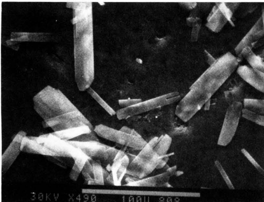
Figure 6. Scanning electron micrographs of solid products from limestone thiosulfate base case test (run LS-0, no thiosulfate addition). (a) Base case; 50x. (b) Base case; 500x.
