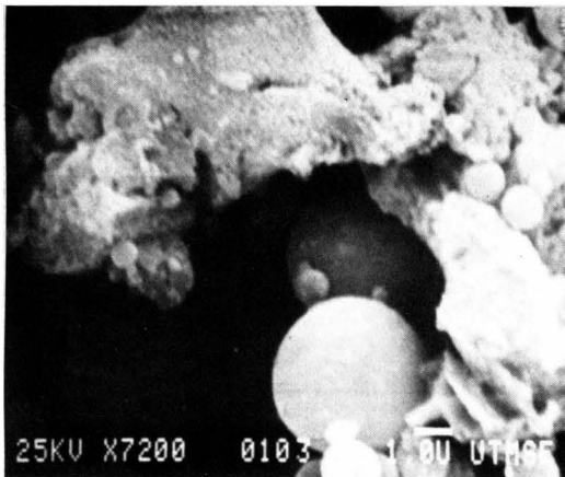
Figure 8. SEM photograph of 16 g fly ash IV/g \text{Ca(OH)}_2 sample slurried for zero hours.
