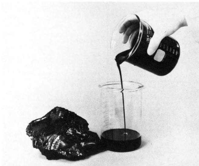
To convert viscous hydrocarbons to usable fuel: A newly patented technology developed by Petroferm Inc. mixes the tar-like heavy hydrocarbon (top center) with a specialty chemicals mixture (smaller beaker top right center) and water (top right beaker), to make Preatomized Fuel™ (PAF™) (bottom beaker), which burns more efficiently and cleaner than No. 6 oil. This is in contrast to current methods which require the use of valuable No. 2 oil mixed with hydrocarbons to make No. 6 oil.
