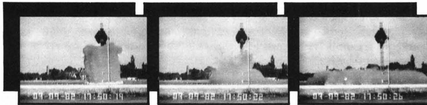
Thorney Island dense gas experiment — time-lapsed over 17 seconds.
