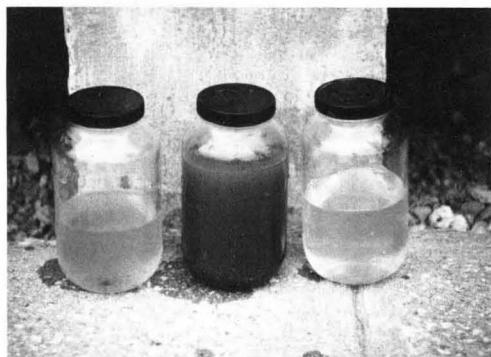
Figure 11. Comparison of overflow samples from baffled and unbaffled paired clarifiers operating in parallel at 28 \text{ m}^3/\text{m}^2 \cdot \text{d} on Little River Pollution Control Plant activated sludge mixed liquor: center = influent mixed liquor; left = overflow from unbaffled clarifier; right = overflow from clarifier equipped with a flow contraction baffle.
