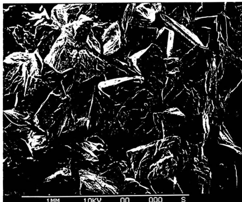
FIGURE 2. Ceramic particles of Kerapak® support. The white line represents 1 mm.
