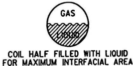
FIGURE 3. Batch reactor design.
