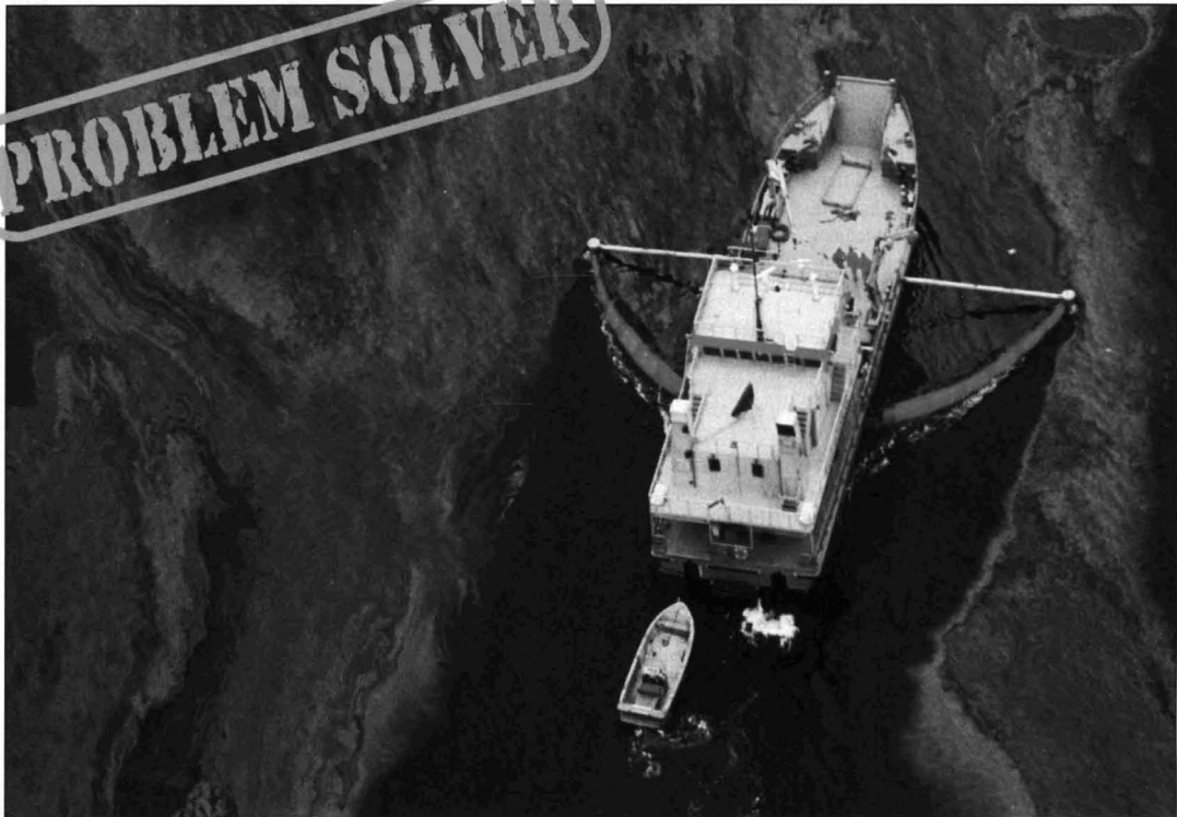
LORS-5 System installed on Swedish Coast Guard vessel during oil recovery operation off the Swedish coast.
