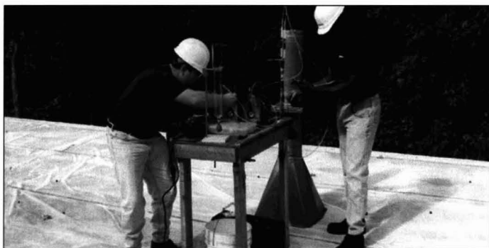
VOC testing at a printing facility using EPA Method 18.
