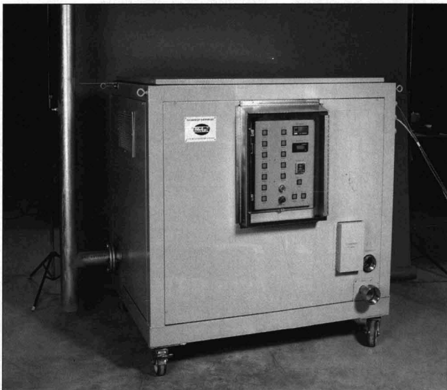
The KSE-developed AIR Process unit used at Dover AFB is pictured above. The unit operated at an average flow rate of 55 SCFM and at conversion levels of 95 percent to 99-plus percent for destruction of total hydrocarbons.
