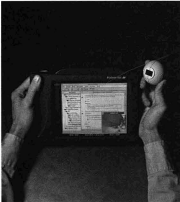
Software such as Dakota Auditor™ is loaded on a portable Fujitsu pen-based computer. Digital images of objects or sites captured by the Connectix camera are incorporated into a draft audit report.
