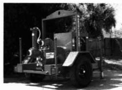
Thompson Pump's new line of compressor assisted pumps features the Enviroclean System, which efficiently handles dry prime applications without any discharge of pumping effluent onto the ground. The system features a mechanical air/water separator device that is installed on a centrifugal pump with an add-on compressor/venturi priming system. Thompson Pump and Manufacturing Co. **Circle 69 on card.**
