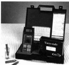
The Ozone Single Analyte Meter uses an LED as a light source and features a long-lasting silicon photodetector. Total analysis time is approximately 2 minutes. Testing range is 0 to 3.0 ppm with a method detection limit of 0.15 ppm. Applications include municipal drinking water plants, wastewater plants and more. CHEMMetrics Inc.
