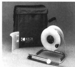
Improvements to the Model KIR Product Interface Probe include auto shut-off circuitry to extend battery life, improved access to the battery for easier replacement and stainless steel wires for increased tape strength. The Model KIR is portable and reel-mounted and has audible and visible indicators. Keck Instruments Inc.
