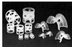
Jaeger Rings are slotted, cylindrical packing elements with standard Pall® ring type dimensions, free space, surface area and performance. Jaeger Saddles have a unique drip-point design that promotes high mass-transfer rates through effective wetted surface renewal. They are available in three sizes—1-inch, 2-inch and 3-inch. Jaeger Products Inc. **Circle 66 on card.**
