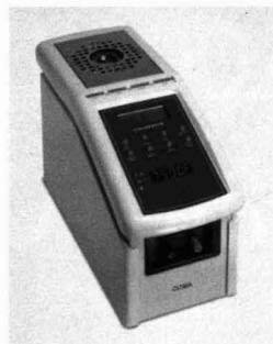
The CL700A series of block calibrators are housed in a rugged metal case for field use. It includes an RS-232 computer interface for data and program transfer or real time control. The calibrators have a fast settling time for rapid testing and fast heat up and cool down times. Omega. **Circle 65 on card.**
