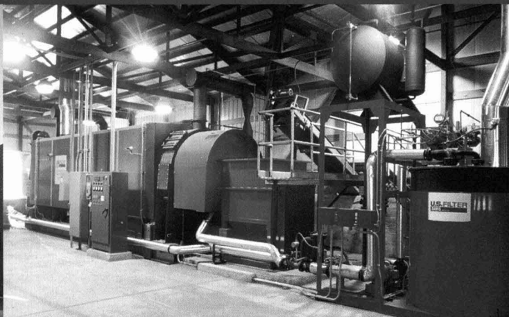
SludgeMASTER® Dryer dehydrates sludge and turns biosolids into a high quality nutrient rich Class "A" soil amendment.
