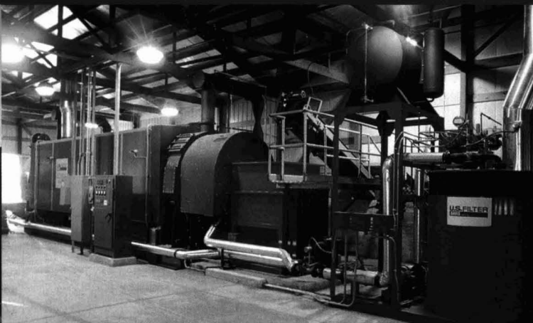
SludgeMASTER® Dryer dehydrates sludge and turns biosolids into a high quality nutrient rich Class "A" soil amendment.
