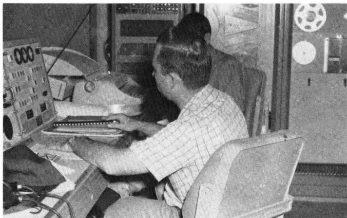
Monitor. The computer control room of the U.S.S. SILAS BENT monitors the output from the electronic salinity-temperature-depth instrument
