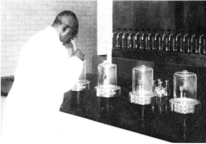
Monitoring. Probably the most widely acceptable method of monitoring the taste and odor quality of untreated and finished waters is with the help of the Baylis nose-piece
