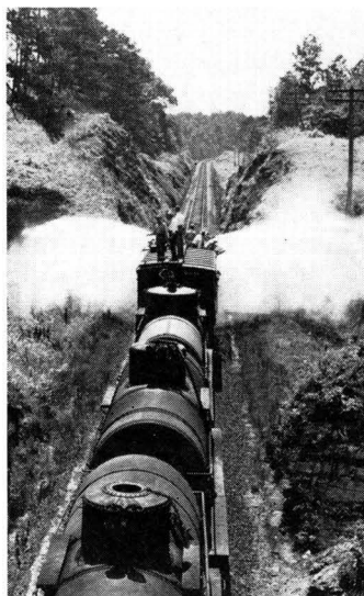
Control. Herbicides are fast replacing such methods for the control of unwanted vegetation as burning, rotary mowing, and hand removal
