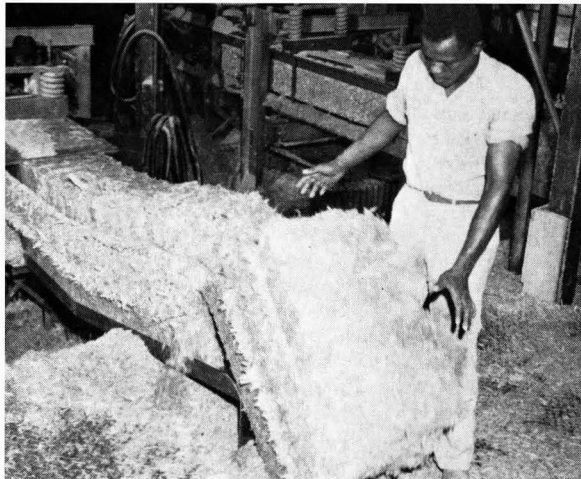
Useful product. Converting processing wastes into commercial products is the ideal solution to waste abatement. Some sugarcane bagasse is used as fuel in the factory, but most is dried, baled, then sold to be made into insulation board
