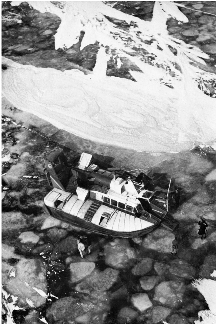
Ice fields. During Lake Erie project, ACV encountered massive ice fields and pressure ridges, but maintained average speed of 30 m.p.h.
