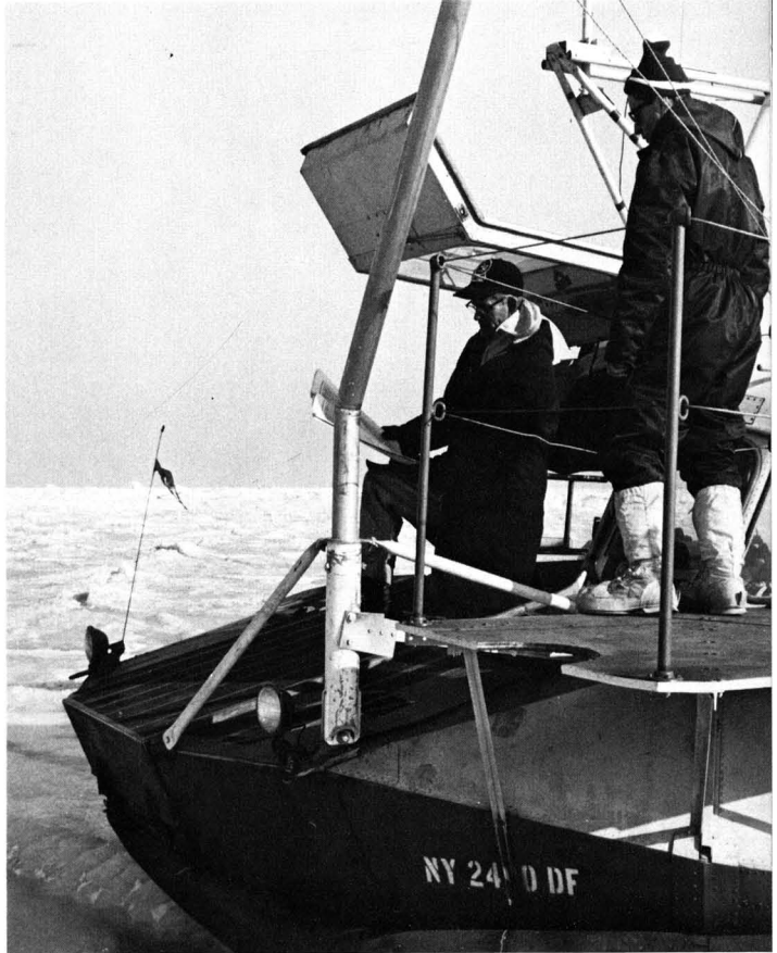
Bow platform. Special platform on ACV facilitated lowering of instruments through the ice cover and recovery of water samples
