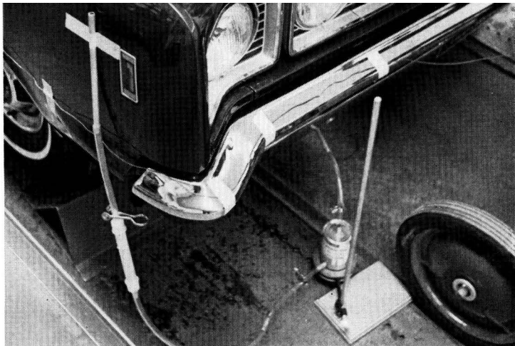
Evaporative losses. Required tests for evaporative emissions control on 1970 and 1971 model vehicles takes 13 hours at Michigan facility
