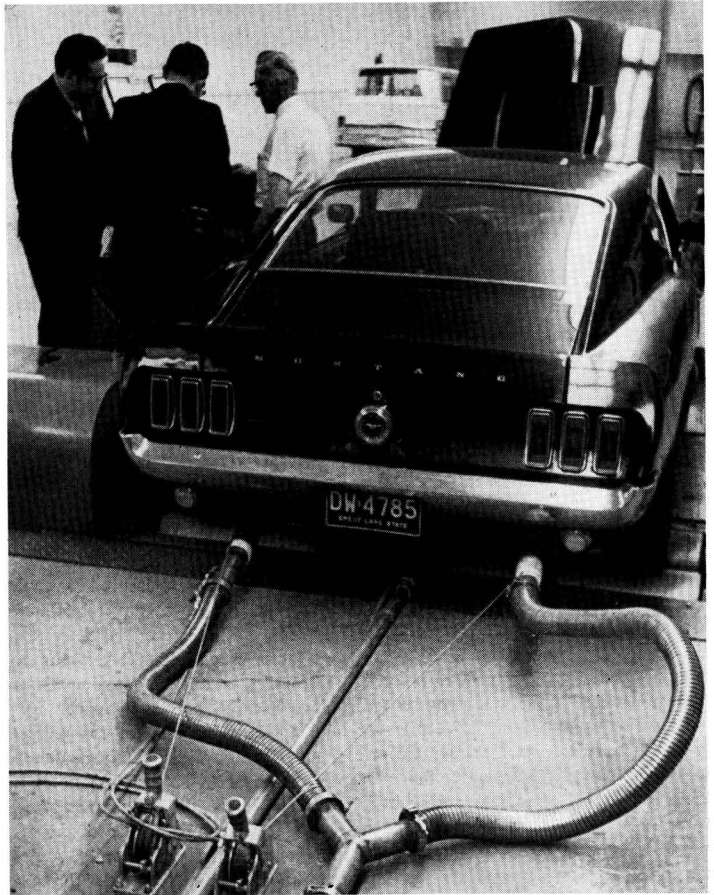
High emissions. NAPCA facility tests vehicles with high performance engines, manual transmissions, and multiple carburetors, which have significantly higher emissions than conventional automatic transmission vehicles
