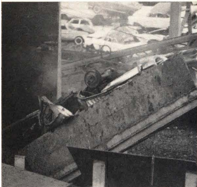
Shredder input-output. A junked automobile (left) is being processed by new shredder; after being cut into sections, these sections are fed into the hammer-mill type shredder (center), which then shreds the hulk into fine pieces of metal (right)
