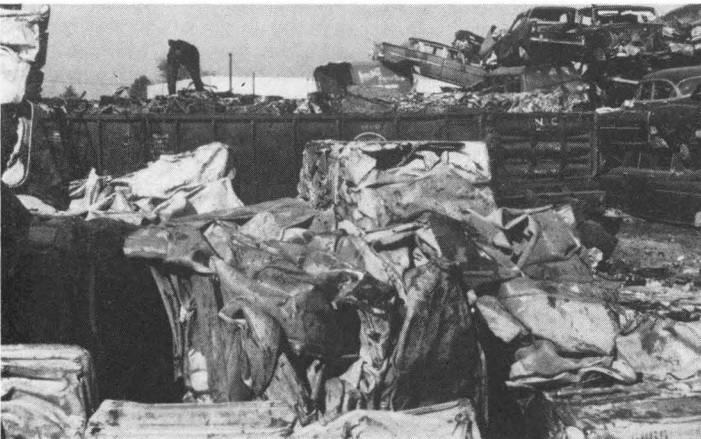
No. 2 bundles. Weighing about 1200 pounds each, this basic auto scrap item accounted for one quarter of domestic steel mills and foundries' purchases in 1967
