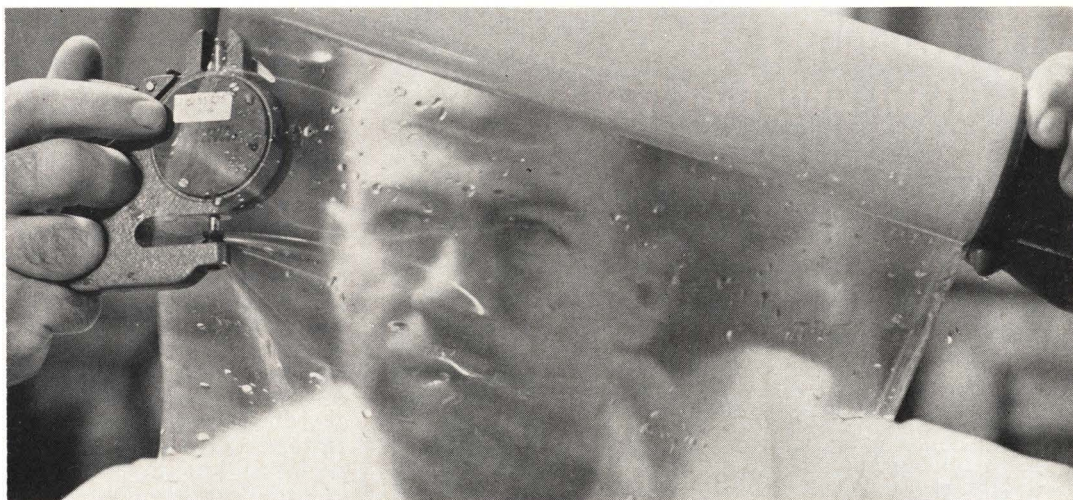
Inspection. Cellulose acetate is a common material for reverse osmosis membranes
