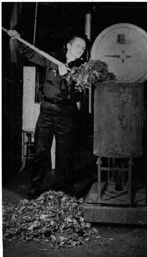
Technician at BuMines' Pittsburgh Energy Research Center charges experimental pyrolysis unit with shredded municipal refuse
