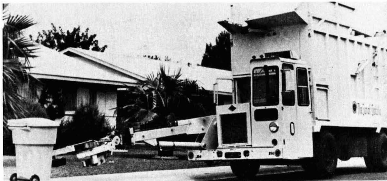
Removal. Automated collection vehicles allow the operator to remain in the cab while picking up containers and dumping the contents into the packer body behind
