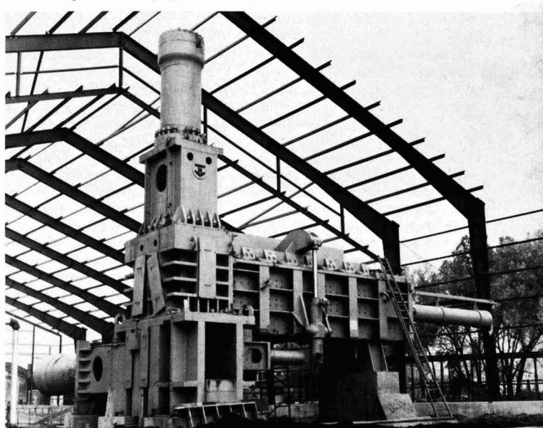
Reduction. Three rams in this baler operate consecutively along three octagonal directions to compress 60 tons of refuse each hour into 2500–3000-lb bales
