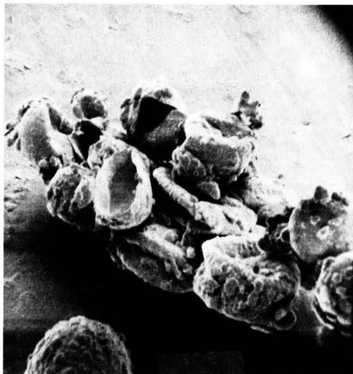
Figure 2. Crushed Freon 113 microcapsules, enlarged \sim 2000 times
