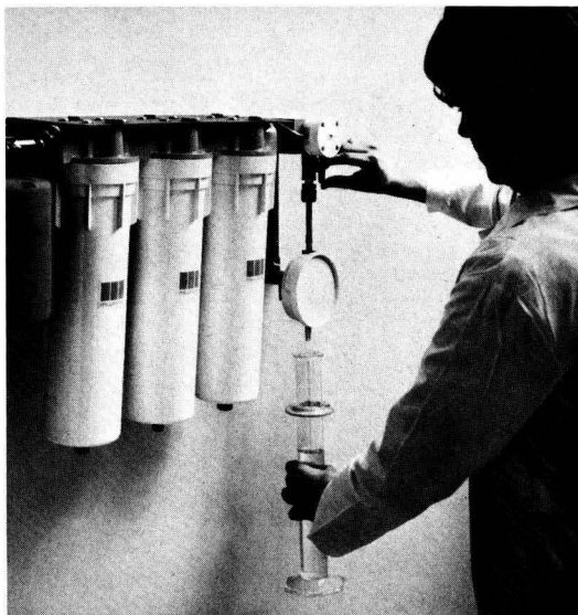
Milli-Q systems can produce reagent grade water at a rate of 1½ liters per minute at a level of purity higher than the highest ASTM and CAP specifications.
