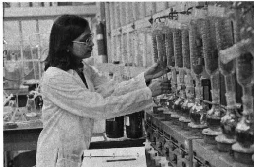
COD digestion. Lab assistant checks on progress of wastewater analyses of samples containing a chemical-oxygen-demand pollutant
