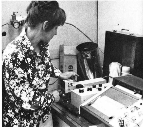
Gas chromatograph. In the laboratory, the analyst injects a sample for plant metabolism studies
