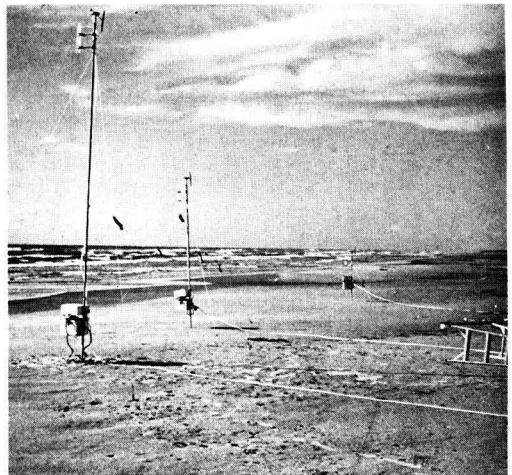
Figure 1. Aerosol samplers at three elevations along a Padre Island beach
