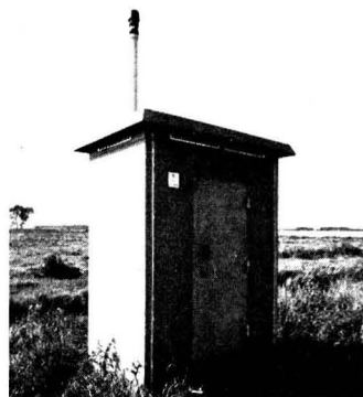
A Philips multi-component air monitor within typical weatherproof housing. This forms part of the Dutch national air monitoring network.
