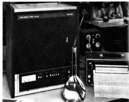
Effluent samples automatically being measured and recorded.
