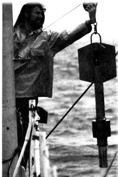
Water sampling. Taking bottom sediment samples from Chesapeake Bay
