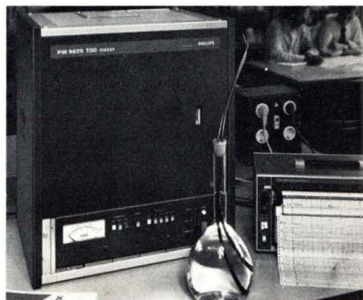
Effluent samples automatically being measured and recorded.
