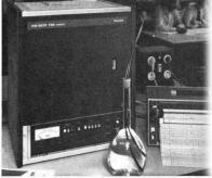
Effluent samples automatically being measured and recorded.
