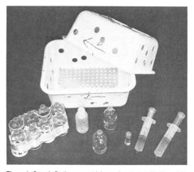
Figure 1. Sample Packages containing various types of bottles, vials, syringes, etc., for in situ incubation of solid and dissolved organic materials on deep-sea moorings at 5300 m depth
