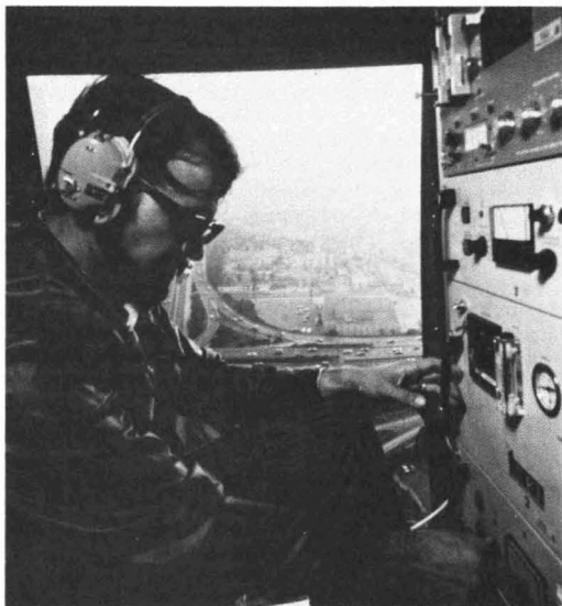
Airborne platforms. This type of monitoring is efficient and cost effective for urban areas and long-range transport studies
