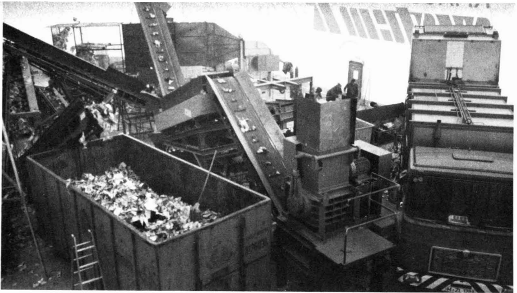
Krauss-Maffei. The pilot system processes 5 tph of refuse to recover paper and metals
