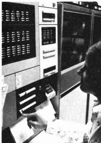
Entering data. Operator assures the required data accuracy with a key-disk system—a Mohawk Data Sciences 2409 System
