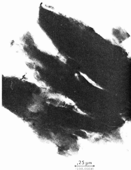
Figure 12. Electron micrograph of carbonaceous reductant from furnace insert D (see Figure 1). Magnification = 100 000X
