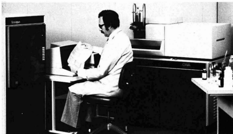
Dedicated instrument. The Organics-in-Water analyzer, a GC/MS system with 9-track magnetic tape drive, can be operated by laboratory technicians after a short training period
