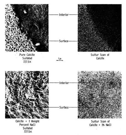
Figure 7. Effect of NaCl treatment on calcination/sulfation of calcite spar at 850 °C for 5 h in 0.3 % SO<sub>2</sub>, 5% O<sub>2</sub>, 20% CO<sub>2</sub>, balance N<sub>2</sub>
