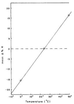
Figure 3. Effect of temperature on rate of permeation
