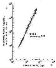
Figure 7. Membrane filter counts vs. sample mass (wet) for 11 strains of bacteria
