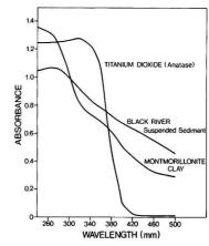
Figure 1. Ultraviolet–visible absorption spectra of TiO₂ (anatase), Black River suspended sediment, and montmorillonite clay
