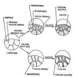
Figure 6. Magnified cross-section comparison of limestone calcination and sulfation, with and without salt (schematic)
