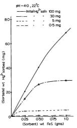
Figure 1. Mercuric ion adsorption on powdered FeS in 500 mL of solution. The time of reaction in each case is 30 min
