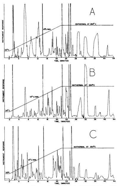
Figure 4. The effect of sample mass on PGLC response, three chromatograms of E. coli ATCC 11303: (A) 196 μg; (B) 174 μg; (C) 52 μg
