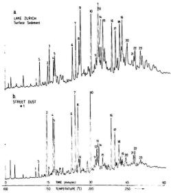
Figure 1. Glass capillary gas chromatograms of nitrogen-containing compounds in Lake Zurich surface sediment and a street dust. Numbers refer to peaks identified in Table III; S = octadecanoic nitrile
