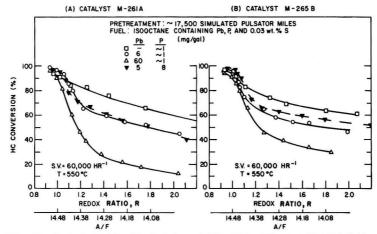
Figure 2. Effects of Pb and P on the steady-state HC activity of pulsator-aged TWCs of different Rh content: (A) M-261A (Pt/Rh = 19) and (B) M-265B (Pt/Rh = 5)
