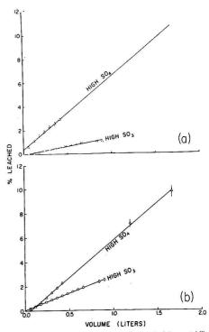
Figure 3. (a) Sulfite + sulfate and (b) Ca leached from stabilized scrubber sludge and fly ash during percolation
