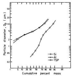
Figure 2. Log probability plot of size distributions for silicon, aluminum, and TSP at Nagoya, May 12-18, 1978. Mass median diameters are 5.7  $\mu$ m (Si), 5.8  $\mu$ m (Al), and 0.68  $\mu$ m (TSP)
