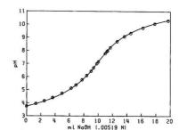
Figure 6. Titration of water from 5% lignite slurry
