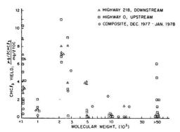
Figure 4. Chloroform yield vs. molecular weight
