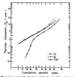
Figure 4. Log probability plot of size distributions for silicon, aluminum, and TSP influenced by Kosa at Nagoya, March 12-18, 1977. Mass median diameters are 4.2  $\mu$ m (Si), 4.0  $\mu$ m (Al), and 2.9  $\mu$ m (TSP)
