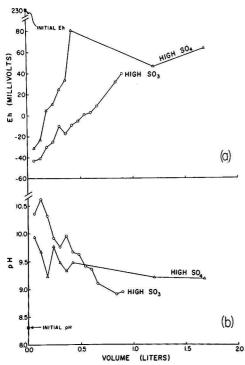
Figure 2. Eh (a) and pH (b) of seawater percolating through test samples of stabilized scrubber sludge and fly ash
