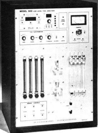
For drinking water • boiler feed · ultrapure compounds and much more. Introducing the Model 600. All new. Faster. Truly automatic. Detection by flame ionization. Unique purge trap system gives separate peaks for purgeable and non-purgeable organics in less than 4 minutes. Direct conversion to methane (no intermediate steps) means vastly superior precision and sensitivity. Send for letailed brochure!
