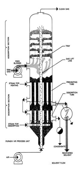
Figure 2—PURASIV® HR Flow Diagram Steam Stripping
