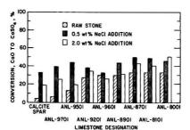
Figure 3. The effect of 0.5 and 2.0 wt % NaCl treatment on limestone subsequently precalcined and sulfated at 850 °C for 5 h in 0.3 % SO<sub>2</sub>, 5% O2, 20% CO2, balance N2
