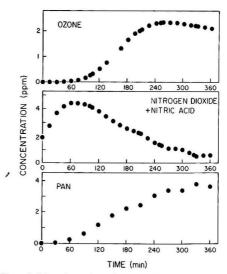
Figure 1. Selected experimental concentration-time profiles for  $\mathcal T$ = 16.1 °C, run no. 193
