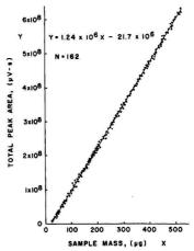
Figure 6. Total peak area of chromatographic signal vs. sample mass (wet) for 11 strains of bacteria
