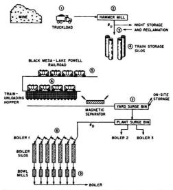
Figure 1. Flow diagram for the mining and handling operations at the Kayenta Mine and the Navajo Generating Station
