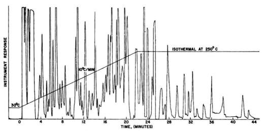
Figure 9. Composite E. coli chromatogram, approximately equal amounts of ATCC 11303 and ATCC 12435
