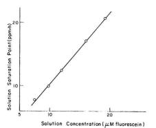
Figure 3. Cl<sub>2</sub> saturation point for absorber solutions
