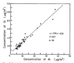
Figure 7. Scatter diagram of silicon and aluminum in aerosols at Nagoya, September 1976–September 1978
