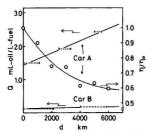
Figure 2. Oil consumption rate (Q) and relative oil viscosity vs. oil mileage. Broken lines: kilometers where oil consumptions were measured
