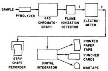
Figure 3. Sample analysis and signal processing schematic
