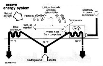
groundwater cooling, computercontrolled waste heat, and chemical dehumidification principles. The complex will house more than 3000 employees. In corridors, sunlight will substitute for artificial lighting, for example. Waste heat will be supplemented by heat pumps. With an average temperature of 59 °F, the groundwater is an effective coolant. Building shaping will also maximize solar use and energy savings.
