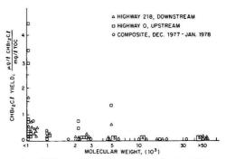
Figure 6. Dibromochloromethane yield vs. molecular weight
