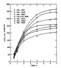
Figure 2. Reaction curves for limestones treated with 2 wt % NaCl, then calcined and sulfated simultaneously at 850 °C for 5 h in 0.3% SO<sub>2</sub>, 5% O2, 20% CO2, balance N2
