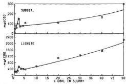
Figure 1. Chemical oxygen demand (COD) as a function of percent coal in subbituminous and lignite slurries
