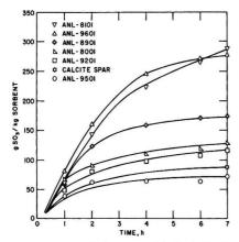
Figure 1. Reaction curves for limestones calcined and sulfated simultaneously at 850 °C for 5 h in 0.3% SO2, 5% O2, 20% CO2, balance No
