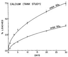
Figure 5. Release of Ca during the tank leaching experiment
