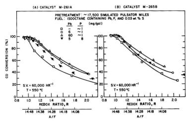
Figure 3. Effects of Pb and P on the steady-state CO activity of pulsator-aged TWCs of different Rh content: (A) M-261A (Pt/Rh = 19) and (B) M-265B (Pt/Rh = 5)
