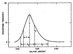
Figure 3. Frequency distribution of mine core percent sulfur showing definition of daily mining range
