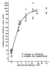
Figure 2. Cumulative percent of TOC less than a given molecular weight, lowa River, Oct 17-Nov 21, 1977
