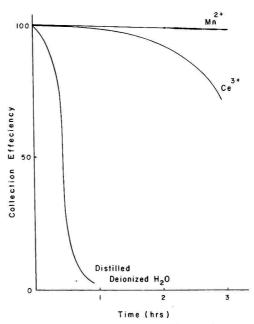
Figure 2. Collection efficiency of 10 ppm of Ce3+ and Mn2+ solutions
