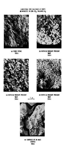
Figure 5. Limestone ANL-9501 calcined at 850 °C for 1 h in 5% O<sub>2</sub>, 20% CO2, balance N2 after treatment with NaCl
