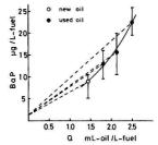
Figure 3. BaP emission rate vs. oil consumption rate for car A
