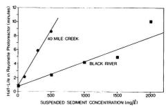
Figure 2. The effect of suspended sediment on the half-life of methoxychlor in a Rayonette photoreactor (wavelength of irradiation, 300 nm)
