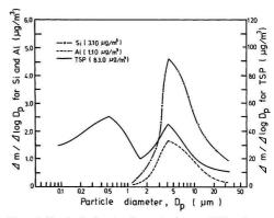
Figure 3. Size distributions for silicon, aluminum, and TSP at Nagoya, May 12-18, 1978
