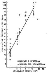
Figure 8. Cumulative percent of total trihalomethanes formed from organics of less than a given molecular weight, October-November
