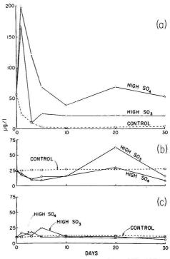
Figure 4. Results from tank leaching experiments: (a) Fe; (b) Cu; and
