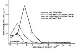
Figure 3. Trihalomethane concentration as a function of precursor molecular weight, Iowa River water, December 1977-January 1978
