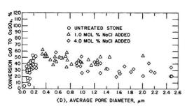
Figure 8. Percent conversion of CaO to CaSO<sub>4</sub> vs. average pore diameter (pores  $\geq 0.3~\mu m)$  for limestones at 850 °C with and without NaCl calcined for 1 h in 5 % O2, 20 % CO2, balance N2, and sulfated for 5 h with added 0.3% SO2
