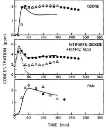
Figure 3. Selected experimental and model calculated concentration-time profiles for T=48.9 to 50.5 °C runs: run no. 209, ( $\blacksquare$ ) experimental; (——) model calculation ( $O_3$ ,  $NO_2$  + HNO $_3$ , PAN); (---) model calculation, NO $_2$  only; run no. 211, ( $\triangle$ ) experimental
