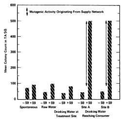
Figure 3. Mutagenicity of chemical concentrates of different waters from water supply CH. Chemicals were recovered from water by sorption on polyurethane foam columns. The data shown represent mutagenic activity with 0.1 mL of concentrate, representing 100 mL of test water/assay. An increase in the number of revertants at distribution sites A and B over drinking water at the treatment site is significant at p < 0.05
