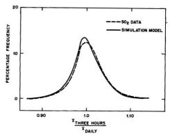
Figure 4. Comparison of observed and predicted distributions of sulfur emissions from the Navajo Generating Station
