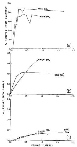
Figure 1. Results from the percolation leaching experiment: (a) Fe removed from seawater; (b) Cu leached from the test samples; (c) Ni leached from the test sample
