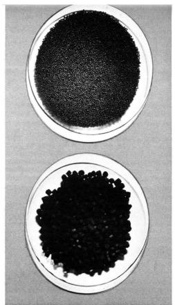
Figure 1—Beaded activated carbon (top) and conventional pelletized activated carbon.
