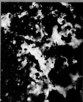
6: Detergent residue. Fluorescence 90x.
