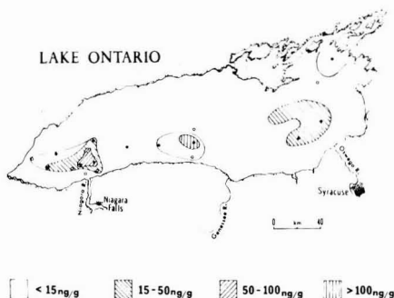
Figure 4. Concentration isopleths of octachlorostyrene in Lake Ontario. Open circles indicate data from grab samples; closed circles indicate data from sediment cores.
