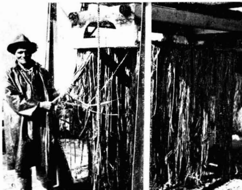
Retted ribbons hanging in fibre glass frames prior to washing
