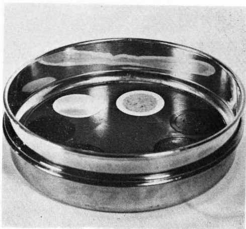
Fig. 3. Final washing of membranes
