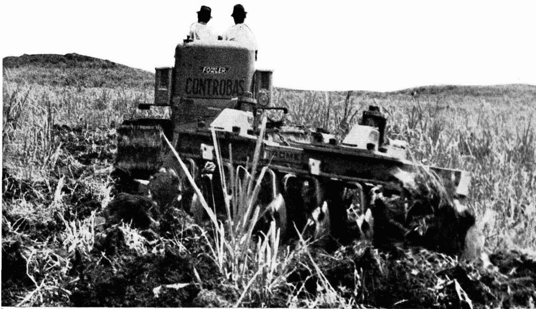
A 125 bhp Fowler Challenger 33 crawler tractor hauling a set of disc ploughs on one of the Azucarera Haina Estates in the Dominican Republic.
