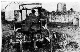
A Track-Marshall crawler tractor fitted with hydraulic toolbar sub-soiling for sugar planting on a sugar estate in the West Indies.
