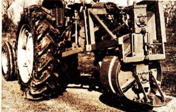
V-DITCHER , for building, cleaning and maintaining ditches, cut to 36" deep, 30" wide, keeps fields level by dispensing soil up to 70". Smaller model cuts 36" deep, 24" wide.
