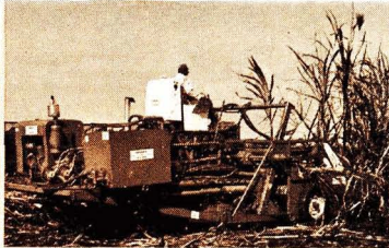
DUNCAÑA HARVESTER , two-row cut-windrow harvester for cane up to 115 tons per acre. Also designed by Richard A. Duncan, world-renowned cane equipment engineer.
