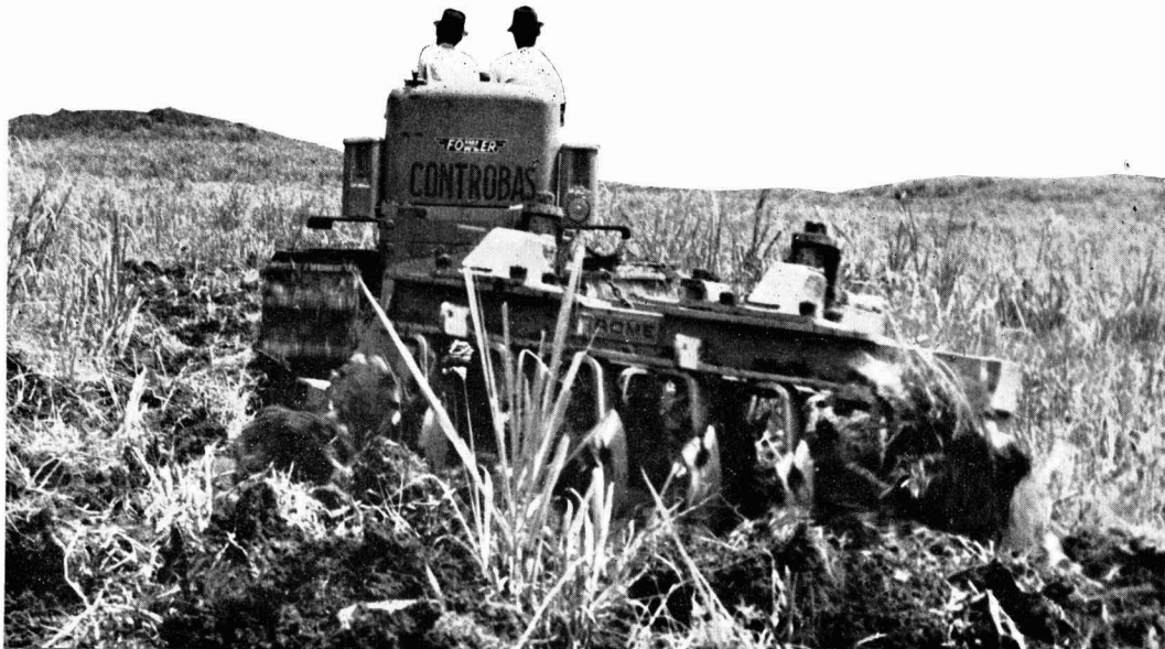
A 125 bhp Fowler Challenger 33 crawler tractor hauling a set of disc ploughs on one of the Azucarera Haina Estates in the Dominican Republic.
