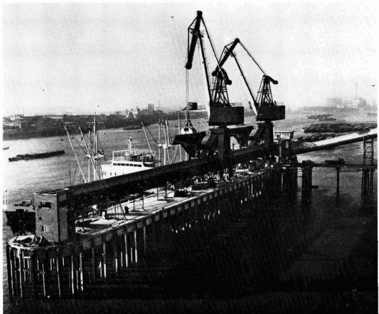
Fig. 3. The jetty section of the bulk sugar handling system at Tate & Lyle Refineries Ltd., London, showing grab cranes of the electro-hydraulic, level-luffing, pantographic type feeding 80-ton capacity retractable hoppers which, with the cranes, travel the full length of the jetty and feed sugar into the conveyor system which delivers it via a junction house and weigh house to the storage sheds.
