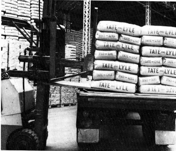
Fig. 4. Palletless loading of bagged sugar using a fork-lift truck fitted with a special carrying plate and push-pull attachment. With this system stacking heights of up to 16½ ft have been attained, with space savings of up to 15%.
