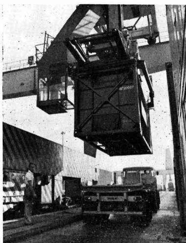
Fig. 2. Tamplin container transfer from road to rail at Stratford Freight Liner Depot
