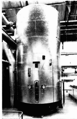
Annular space overflow evaporator
