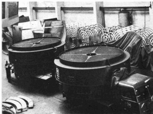
3. Evaporator calandrias of 1600 sq.m. heating surface for Iraq.
